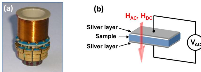
Figure 4. (a) The sample puck for ME measurements ; (b) schematic view of the ME measurement circle
